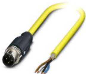
Sensor/actuator cable, 4-position, PVC, yellow, shielded, Plug straight M12 SPEEDCON, A-coded, on free cable end, cable length: 2 m
