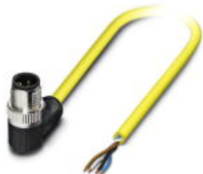
Sensor/actuator cable, 4-position, PVC, Plug angled M12 SPEEDCON, A-coded, on free cable end, cable length: 2 m
