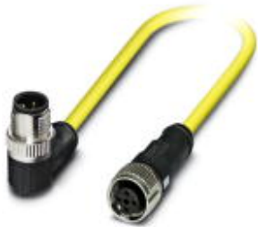
Sensor/actuator cable, 4-position, PVC, yellow, Plug angled M12 SPEEDCON, A-coded, on Socket straight M12 SPEEDCON, A-coded, cable length: 3 m
