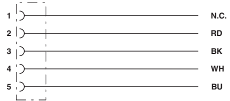
Contact assignment of 7/8" socket
