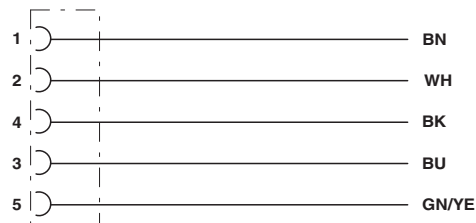
Contact assignment of the M12 sockets
