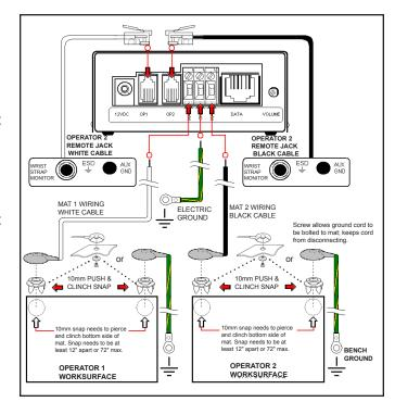
Figure 3. Installing the Dual-Wire Dual-Operator Programmable Monitor
