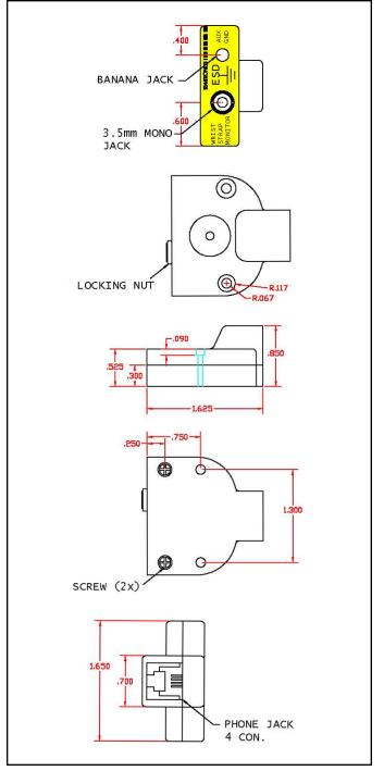
Figure 7. Operator Remote dimensions
