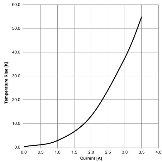
CHECKED GENERAL TOLERANCE PROJECTION METHOD CREATED Würth Elektronik eiSos GmbH & Co. KG EMC & Inductive Solutions KaS CSo DIN ISO 2768-1m Max-Eyth-Str. 1 74638 Waldenburg **WE-WPCC Wireless Power** Tel. +49 (0) 79 42 945 - 0 **Charging Transmitter Coil** ORDER CODE www.we-online.com 760308101105 eiSos@we-online.com DATE (YYYY-MM-DD) BUSINESS UNIT REVISION STATUS PAGE 001.001 2017-04-24 3/6 Ø 20 Valid **WÜRTH ELEKTRONİK**
