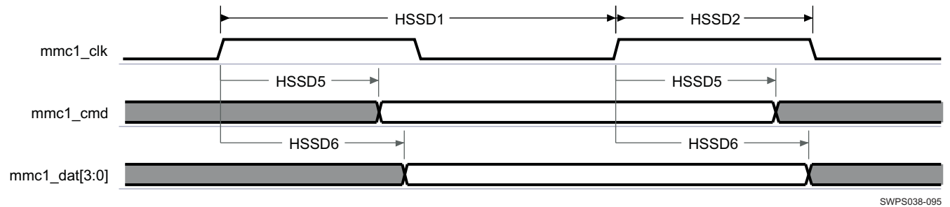
Figure 6-66. MMC1 Interface—High-Speed SD Mode—Data/Command Transmit
