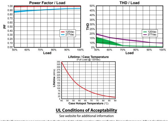
**Note:** The area under the life-temperature curve represents where the driver has highly reliable operation within specification. Driver performance may drift out of published specifications as the hours of operation exceed the curve at a given temperature. Higher operating temperatures increase the chances of a failure to function. Other electrical, mechanical and environmental factors affect driver lifetime but are not represented in this calculation.
