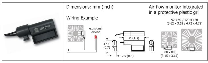
The air-flow monitor provides a simple alternative to indicate positive or negative air flow of fans or blowers. When properly installed and connected in series with an optical (i.e. LED) or audible signaling device, a bi-directional switch will activate an electrical contact if the air flow of the fan falls below 8.2 ft/s, turning the signaling device on or off. The AFM monitor can also be attached to an existing plastic grill or guard.
