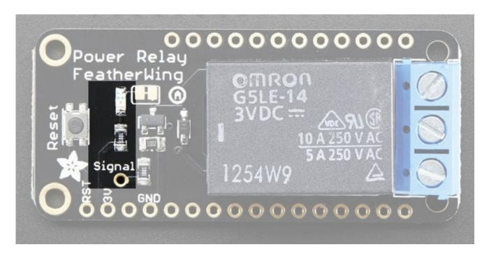
Controlling the relay is really simple. The relay uses a single pin for control. When floating
