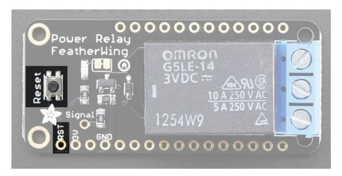
There is a Reset button on both Wings, this is connected to the **RST** pin and will short it to ground. It is not connected to the relay at all, its handy for restarting your Feather
