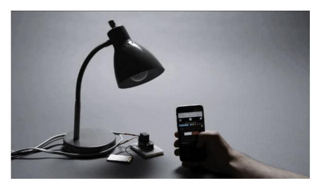
A Feather board without ambition is a Feather board without FeatherWings! This is the **Power Relay FeatherWing**. It gives you power to control, and control over power. Put simply, you can now turn on and off lamps, fans, solenoids, and other small appliances that run on up to 250VAC or DC power using any Feather board. Compared to our smaller mini Relay FeatherWings (http://adafru.it/xDL), this one can handle a beefy 1200 Watts!
