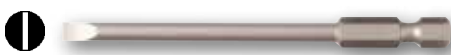
760 Slotted Power Blades S2 modified tool steel. Hardened & tempered to HRC 60. Blades fit CentroFix power blade handle. OAL 90mm/3.5".
