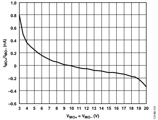
Figure 41. I_{MO+}/I_{MO-} vs. V_{MO+}/V_{MO-} with V_{CC} = V_{MO+} = V_{MO-}
