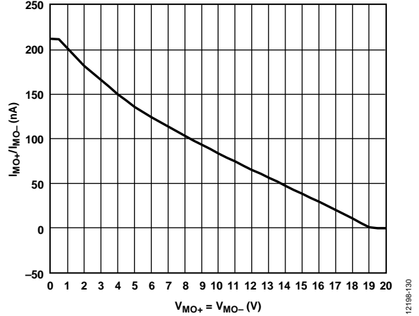
Figure 40. I_{MO+}/I_{MO-} vs. V_{MO+}/V_{MO-} with V_{CC} = 20 V
