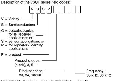
Example: VSOP38336 = receiver chip with  $f_0 = 36$  kHz
