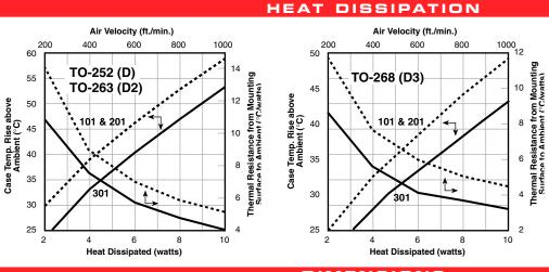
Final thermal performance is highly dependent on the thermal characteristics of the PCB. It is possible to see a 50% drop in temp rise in natural convection with a thermally improved PCB.
