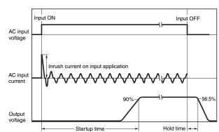
**Note:** Twice the input current or above will flow during the parallel operation or redundant system.
