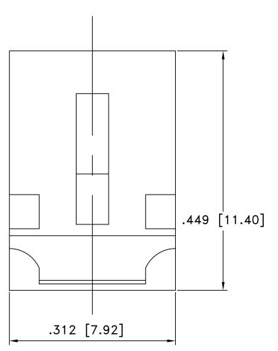
MATERIAL: 0.012" SPRING STEEL, NICKEL PLATED ROHS 2 COMPLIANT
