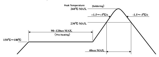
Note 1 Temperature Profile for the reflow soldering is listed as the temperature of resin surface. This represents the maximum temperature ratings for soldering. Lowering the heating temperature and decreasing heating time is very effective in ensuring higher reliability.
