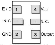
Terminations as viewed from the Top NOTE: XPRESSO HCMOS XOs are designed to fit on Industry Standard, 4 pad layouts
