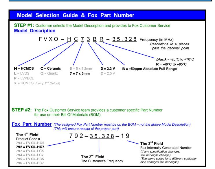
This example, FVXO-HC73BR-35.328 = Voltage Controlled, HCMOS Output, Ceramic, 7 x 5mm Package, 3.3V, ±50 PPM Absolute Pull Range, -40 to +85°C Temperature Range, at 35.328 MHz
