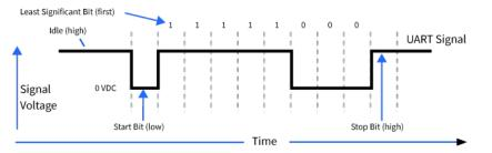
Serial communications depend on the two UARTs (the microcontroller and the RF device) to be configured with compatible settings, including baud rate, parity, start bits, stop bits, and data bits. The UART baud rate and parity settings on the XBee module can be configured with the BD and NB commands, respectively. For more information, see AT commands.
