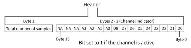
Sample data follows the header and the channel indicator frame determines how to read the sample data. If any of the DIO lines are enabled, the first two bytes are the DIO sample. The ADC data follows. ADC channel data is represented as an unsigned 10-bit value right-justified on a 16- bit boundary. The following figure illustrates the sample data bits.
