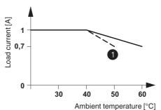
1 For input voltages of 220 V DC and 230 V AC
