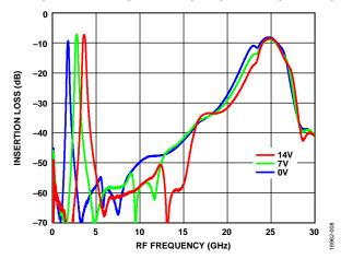
Figure 8. Insertion Loss vs. Broadband RF Frequency at Various  $V_{\text{FCTL}} = V_{\text{BWCTL}}$ Voltages
