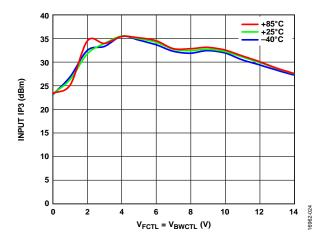
Figure 24. Input IP3 vs.  $V_{FCTL} = V_{BWCTL}$  at Various Temperatures, Input Power  $(P_{IN}) = 20 \text{ dBm}$
