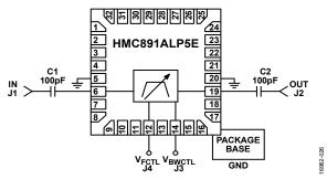
Figure 26. Typical Application Circuit
