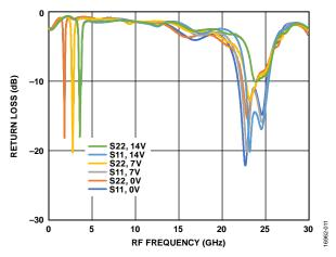
Figure 11. Return Loss vs. Broadband RF Frequency at Various  $V_{FCTL} = V_{BWCTL}$ Voltages
