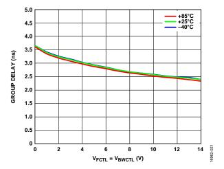
Figure 21. Group Delay vs.  $V_{FCTL} = V_{BWCTL}$  at Various Temperature
